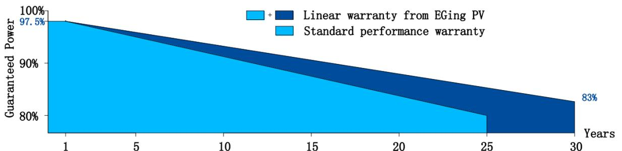
(4) For Monocrystalline double glass modules: not exceed 2.5% degradation in the first year, and 0.5% per year thereafter, ending at 83% in the 30th year after warranty start.
