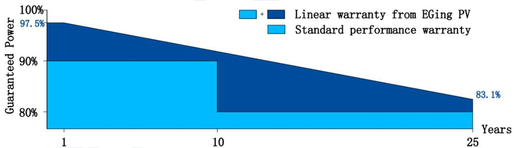
(3) For Polycrystalline double glass modules: not exceed 2.5% degradation in the first year, and 0.5 % per year thereafter, ending at 83% in the 30th year after warranty start.
