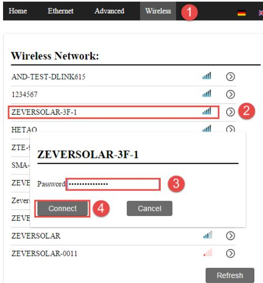
Fig. 5-12 connecting to wireless network
