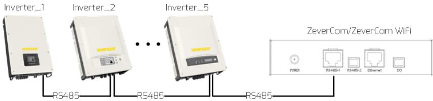
Fig. 5-2: Connection to the inverter
