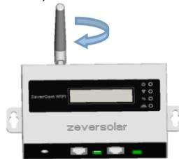
Fig. 4-1: Assemble the antenna
